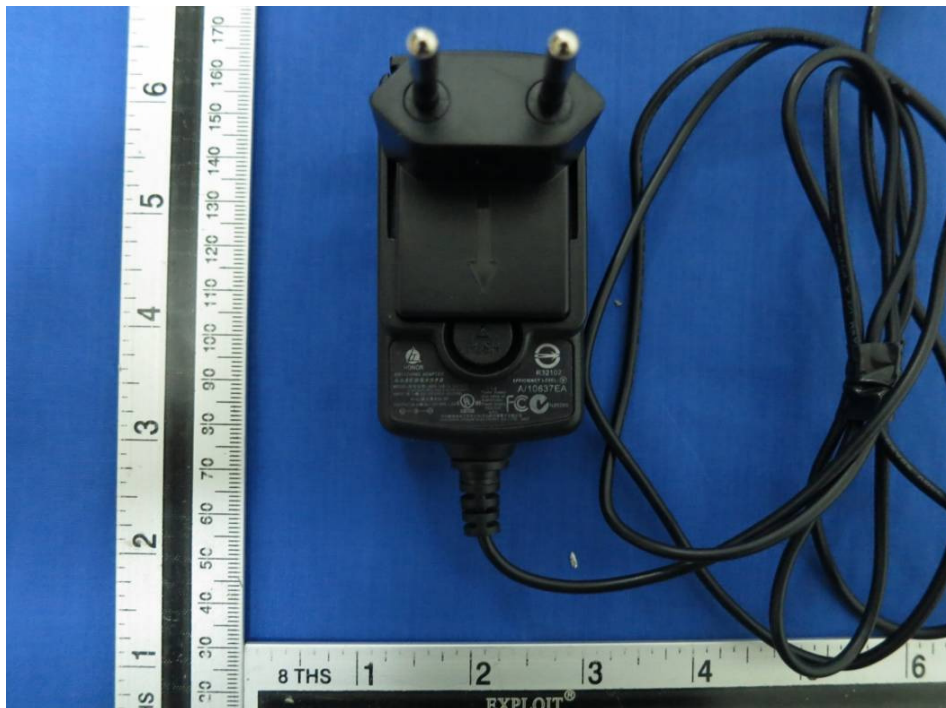
Adapter (Manufacturer: Shenzhen Honor Electronic, Model: ADS-12B-12 12012G)
